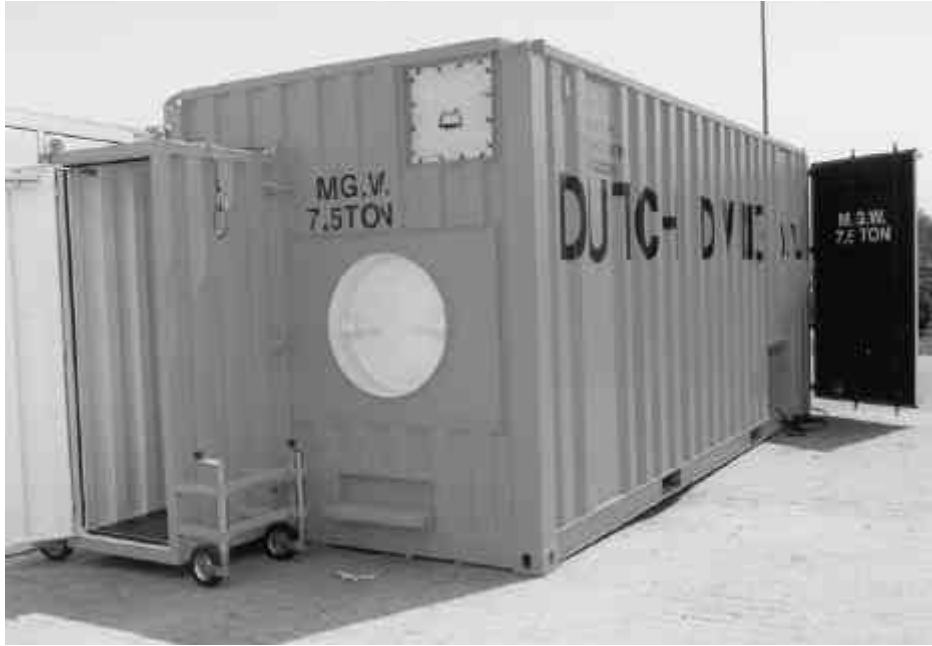
Containerized deco-tank, with skid mounted high pressure air bank, and filter for the low pressure breathing air supply.
