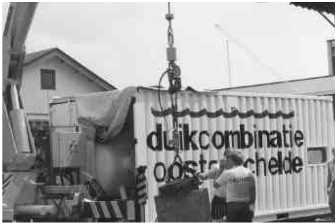
Diving container mounted on a skid with a hydraulic crane, for handling of diving bell.
