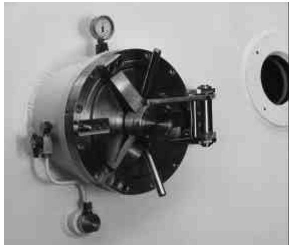
Large size medical lock, with safety interlock system and quick acting door.
