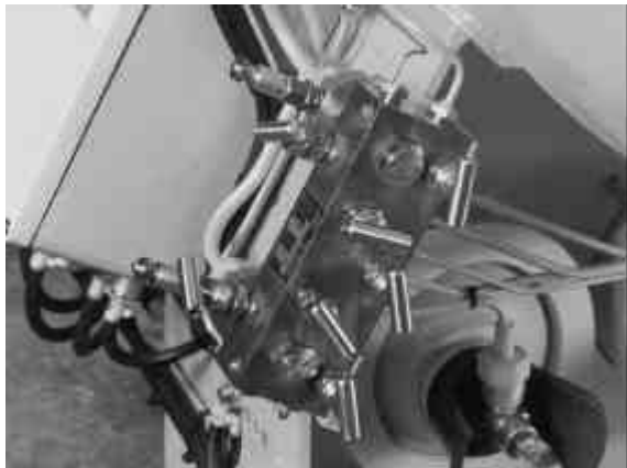
HP-air reducing manifold, made of aluminium bronze.
