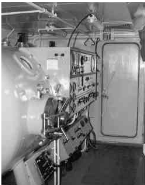
Decompression chamber with medical lock
